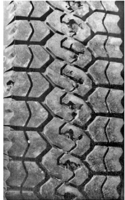
Example of Dyno Damage
