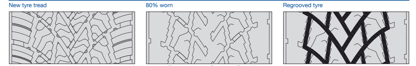
Maximum regrooving depth 3 mm, regrooving width 6-8 mm. Retreadable by Goodyear TreadMax.
