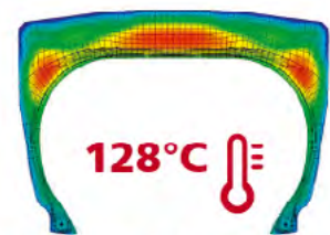
MICHELIN® X MINE® D2 SR at 10 km distance per hour
